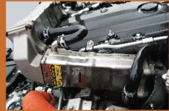
EGR廢氣再循環裝置 (Exhaust Gas Recirculation)
