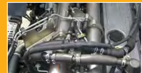
EGR廢氣再循環裝置 (Exhaust Gas Recirculation)
